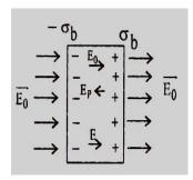
Suppose a dielectric slab is placed in a uniform electric field  $\overline{E_0}$
