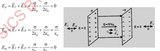
Thus, Electric field is uniform between two plates carrying equal and opposite charge and is directed from positive to negative plate. Outside the plate electric field is zero.
