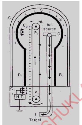
It is a man made high voltage generator. It's a device which produces a high potential difference of about 10 million volts and it can be used as an accelerator of charged particles.
