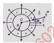
It is to be noted that the field outside a uniformly charged conducting sphere is the same as if whole of the charge was concentrated at the centre of the sphere.
