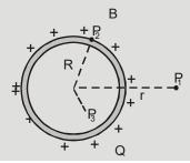
It is constant inside the shell (same at all points inside the shell, as on the surface)
