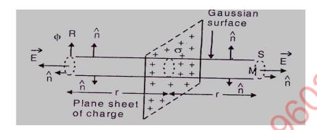
Assuming the cylinder as the Gaussian surface, by symmetry, the electric field on either sides of the sheet should be normal to the plane of sheet, having same magnitude at all points equidistant from
